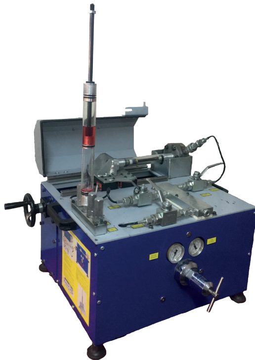
Nitrogen Gas filling from tube side Valve
